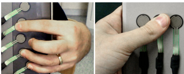
Figure 7: Demonstration of front and rear views of a 5+3 playing configuration for the non-preferred hand controller, with a typical hand position.
