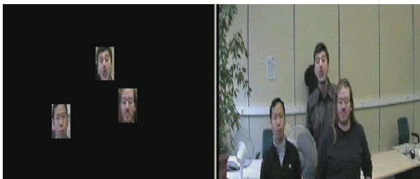
Figure 7: Face detection block implemented in EyesWeb.
