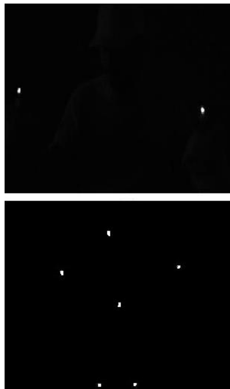
Figure 1: Background subtraction with two blobs (above) and six blobs (below).
