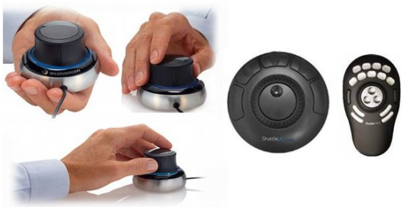
Figure 5: Gestural controllers chosen to be tested in AudioCycle: 3D mice on the left and jog wheels on the right
