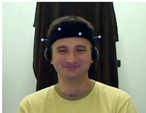
Figure 4: OptiTrack - 23 face markers and 4 head markers on the subject
